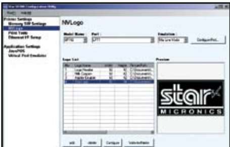
Incorporates futurePRINT™ software with a variety of tools, including the Serial / Parallel Virtual Port Emulator, Graphics Management Tools, as well as Installation and Hex Dump Tools
